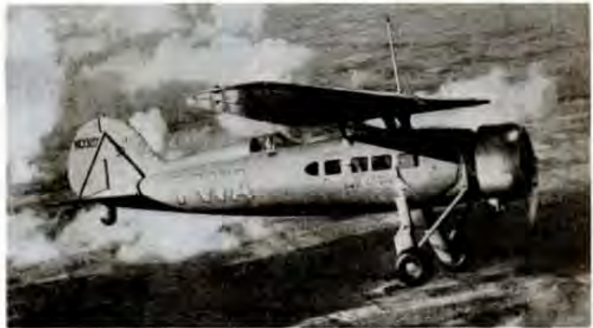
The Transcontinental Fleetster is a unique type of monoplane transport because of its parasol type wing.
